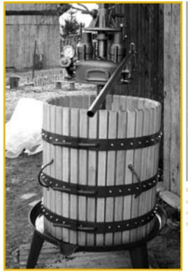
Pressing the juice under the pressure of 400 atmospheres, the juice press is providing a nearby facility for orchard owners to press their apples.
